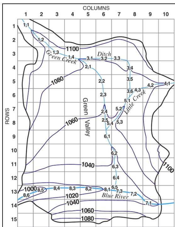
Figure 1 An SFR1 stream network. (Prudic, et al., 2004)
